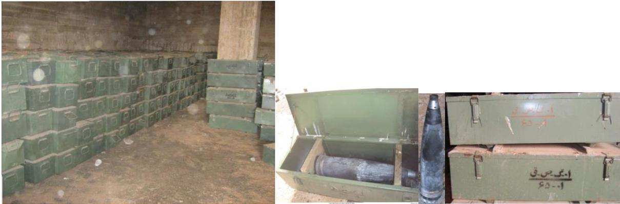
Photographs of the 517 130-mm artillery shells declared by Libya. The Persian markings on the cases (inset) translate to 01-G-S-Gh (meaning unknown) and 65-01 (likely a manufacture date of Farvardin 1365, corresponding to March/April 1986).
