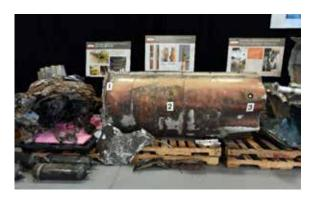
Debris from an Iranian Qiam SRBM provided by Iran to the Huthis that was fired into Saudi Arabia on display at Joint Base Anacostia-Bolling in Washington, DC. The numbered placards identify the unique positioning of valves on the missile's propellant tanks.
